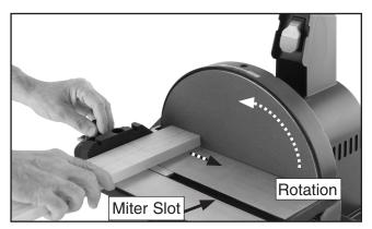
Figure 14. Miter slot and work path.
